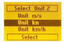
By subsequently pressing switch to "1", units are changed in the following order: m/s, kn, km/h, and mps. New unit is shown in the inverse mode. If you want to select it, press switch to the "0" position. New wind speed unit is permanently stored to the EEPROM; anemometer shows wind speed in these units, until different one is selected.
