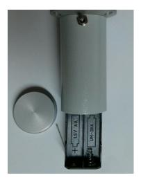
New batteries are able to drive the instrument for approximately 60 hours of continuous use. When the battery voltage falls to the approximately 3 V, the wind-speed section of the instrument ceases to work and **Low Battery** sign is displayed. This indicates that the batteries should be replaced.
