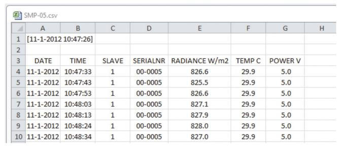
Together with the Modbus® address and the radiation data the body temperature and the power supply voltage to the SMP pyranometer are recorded.
