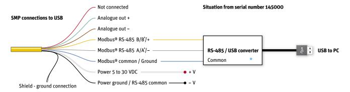
\*Note Switches on the converter should be set for RS-485, 2-wire operation and Echo off.
