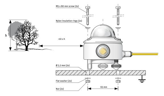
Note After recalibration and/or reinstallation ensure that the nylon insulators are refitted.
