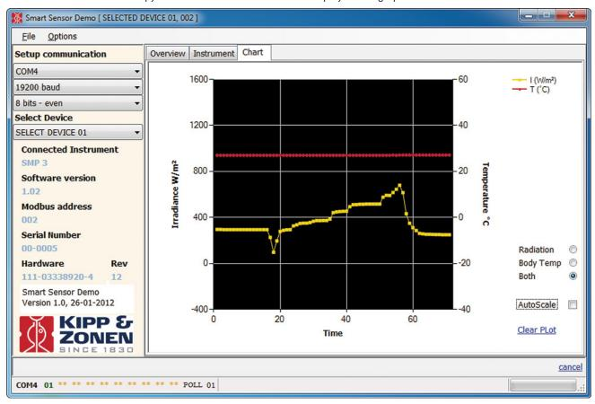
It will show the last 250 measurements of irradiance ('Radiation' in W/m²) and/or the pyranometer housing temperature ('Body Temp' in °C), as an accumulating graph. Vertical scaling can be set to maximum or automatic.
