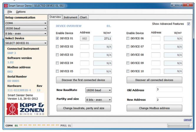
The default Modbus® address of all SMP pyranometers is 1. Before you can use the instrument in your network you must reconfigure the address to a unique number. Each Modbus® device connected to a network must have a unique address.
