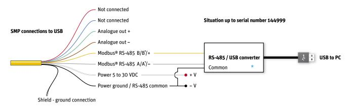
\*Note Switches on the converter should be set for RS-485, 2-wire operation and Echo off.
