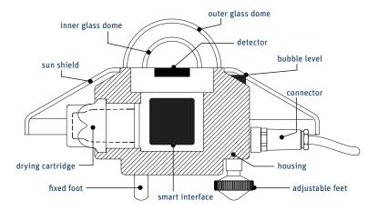
A drying cartridge in the SMP11 radiometer housing is filled with replaceable silica gel and prevents condensation on the inner sides of the domes, which can cool down considerably on clear windless nights. The SMP3 has a sealed construction with a non-replaceable internal drying cartridge.
