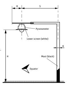
As a guide, a black shadow below the pyranometer with a radius of  $0.1 \times H$  decreases the signal by 1%, and 99% of the signal will originate from an area with a radius of  $10 \times H$ .
